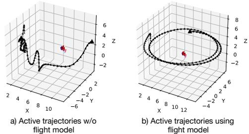
Figure 2. **The trajectories drawn by our active decision making policy** (a) without using our flight model and (b) using our flight model. We are able to find the well performing policy of constant rotation when we are using more realistic sampling of future drone positions, found using our drone flight model.
