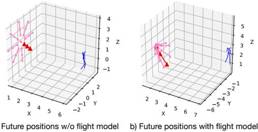
Figure 1. **The predicted future positions of the drone** (a) without using our flight model and (b) using our flight model.
