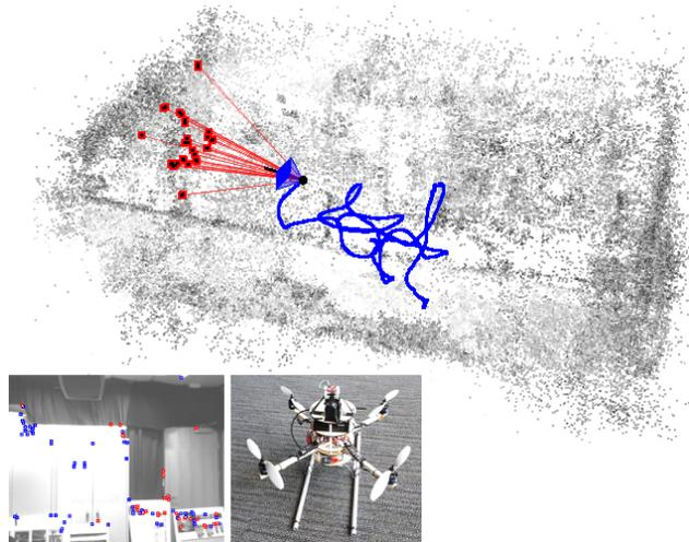
Figure 1: Our method can precisely localize a camera in real-time within a scene reconstructed offline using Sfm. The flight path of a quadrotor micro aerial vehicle (MAV) within a  $8\text{m} \times 5\text{m}$  room (reconstruction has 76K points), and 3D points that were matched to 2D features in the current frame (LOWER-LEFT), are shown.
