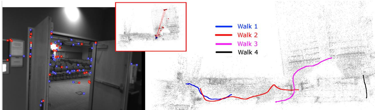
Figure 5: HALL-WALK SEQUENCES: [LEFT] A frame from the WALK3 sequence and the corresponding camera pose estimate shown in the top-view of the map (inset). [RIGHT] Computed trajectories of the camera in the corridor (WALK 1–2), and entering the room through different doors (WALK 3–4). Our approach worked well in this scene despite the presence of many ambiguous and confusing features.
