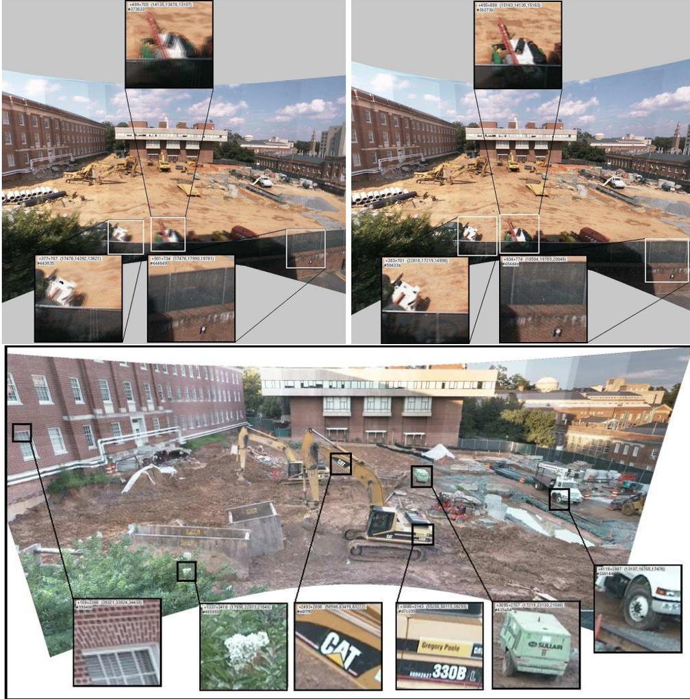
Fig. 8. The front face of the computed cube-maps: (a) Radial distortion was ignored in the camera model (Note that straight lines in the world are not imaged as straight lines). (b) Accurate panorama created after incorporating radial distortion. (c) Part of a high-resolution panorama ( $6000 \times 6000$  pixels) built from 119 images at 5X zoom. Note the zoomed-in regions of the panorama, displayed in the original scale.
